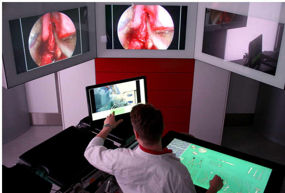
Fig. 2 Demonstration of the trainer system in the demonstration OR at ICCAS. Here, the endoscope screen has been replaced by a connection to the OR monitor matrix
