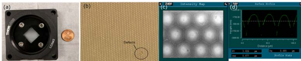
Fig. 5. Lenslet array mount and the characterization of the lenslet array surface. Fig. (a). Photograph of the lenslet array in the rotation mount. Fig. (b). Photograph of the lenslet array through a stereomicroscope. Missing lenslets and defects can be seen and are easy to spot through the stereomicroscope. Fig. (c). Intensity map of lenslets taken with a white light interferometer. Individual lenslet dents and imperfections can be seen. Fig. (d). The surface profile acquired with the white light interferometer. Due to the lenslet curvature, the surface profile is incomplete for steep portions of the lenslets' surfaces.
