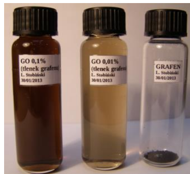
Figure 3 : One of the principal differences, Graphene is hydrophobic, while GO is hydrophilic. (12)
