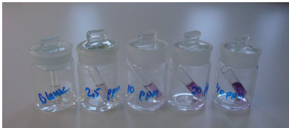
Figure 8. Standard solutions of formaldehyde used for comparison in the chromotropic acid method.
