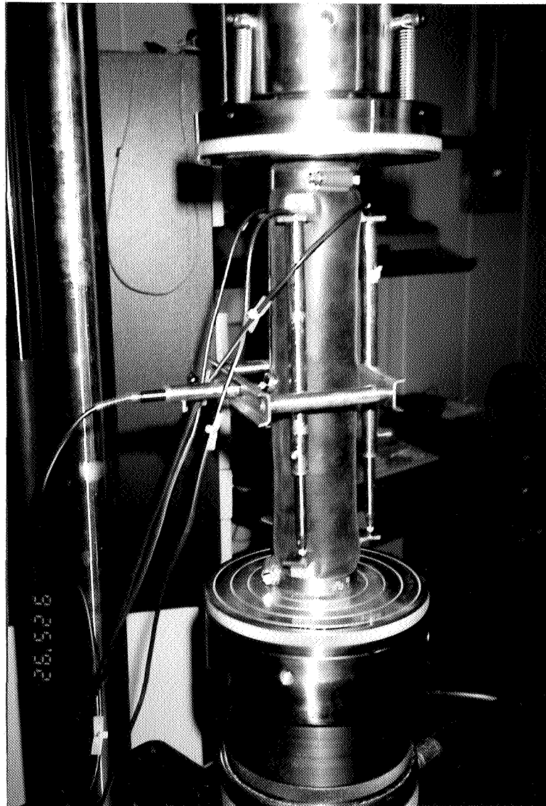
Figure 1. Specimen used in the quasi-instantaneous and short-term creep studies [3].
