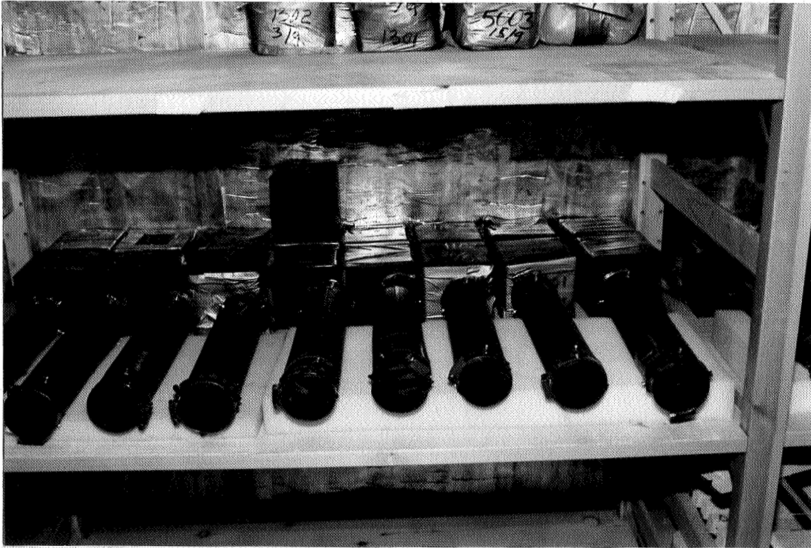
Figure 3. Specimens for studies of autogenous shrinkage. Cubes for strength tests.
