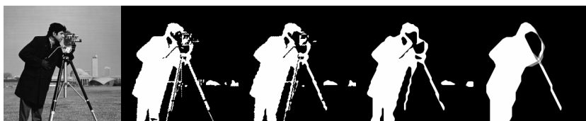
Figure 10.6: Input image and results with a 16-connected 64 \times 64 mesh, using the same parameters as in Fig. 10.4. The solution for \sigma = 10^6 is fractional, as shown by the gray regions.
