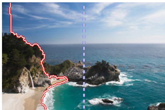
Figure 7.8: “Worst-case” test. The left and right side of the image is connected to the source and sink, respectively. The edge costs are determined by the image gradient. The entire flow must be communicated between the two computational threads when splitting the graph vertically.
