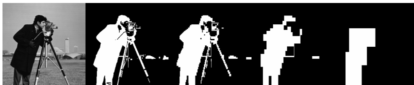
Figure 10.4: Input image and results with regularizations \rho = 100 and \sigma \in \{1000, 10000, 100000, 1000000\} . The mesh is 4-connected of size 256 \times 256 (corresponding to the image pixels).
