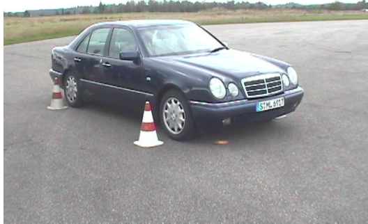
Figure 2.4 The \mathcal{H}^2C test vehicle. It is a modified Mercedes E220 passenger vehicle, fitted with an advanced brake-by-wire system and four state of the art electro-mechanical disc brakes.
