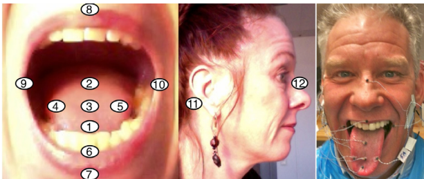
Figure 1: The twelve sensor positions recorded, and one speaker with the sensors attached.
