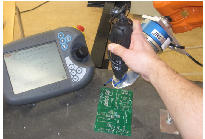
Fig. 6. Physical testing of the drilling skill with manual guidance (force-controlled motions) implemented as a real-time extension with 4ms sampling rate. Boundary conditions are evaluated by calling the corresponding C code.
