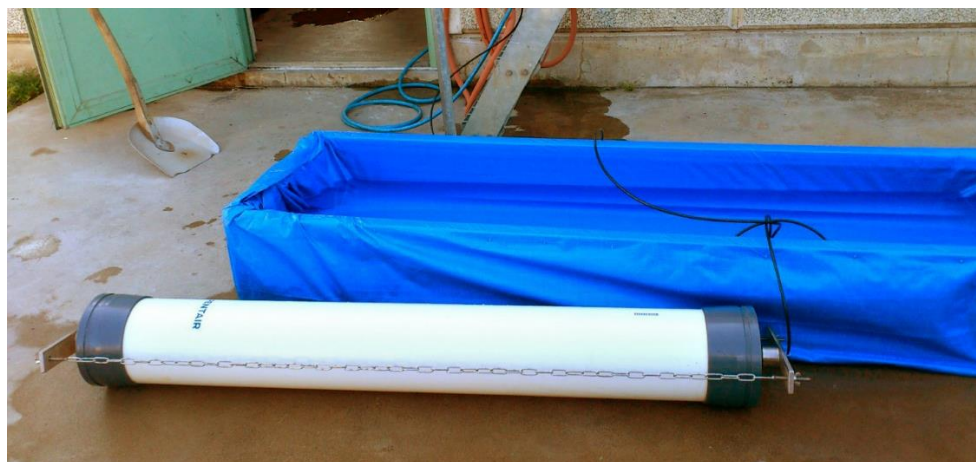
Figure 5 The setup for a bubble point test. The membrane was submerged into the blue box, containing water deep enough to cover the whole membrane.
