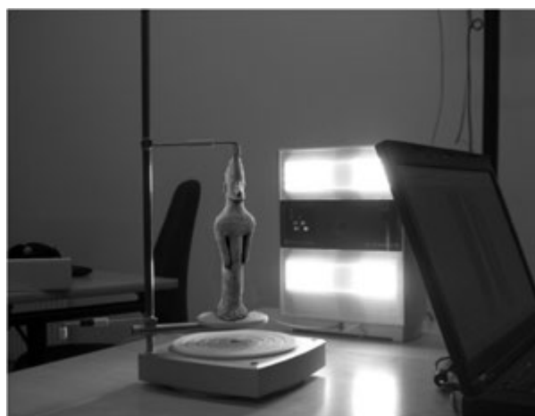
FIG. 3. DATA ACQUISITION OF A TERRACOTTA WITH NEXTENGINE 3D DESKTOP LASER SCANNER.
