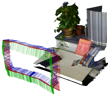
Figure 3.9: Looking at the trajectory and the quality of the 3D model, it is apparent that there is little drift in this sequence.
