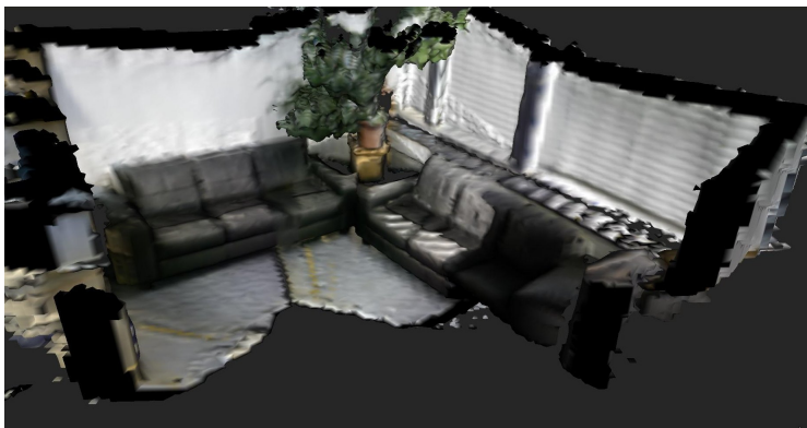
Figure 3.12: Side view of the resulting 3D reconstruction of a room using the assisted mode on the quadcopter.
