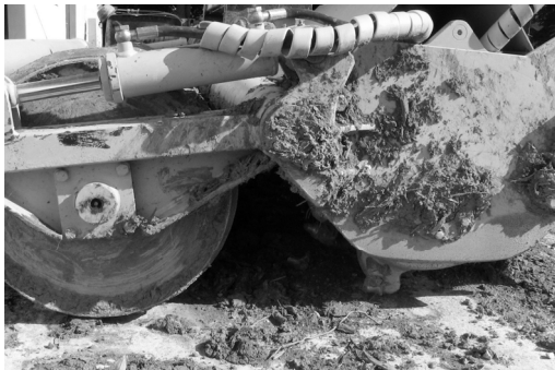
Figure 25. Side View on the Crushing Implement
