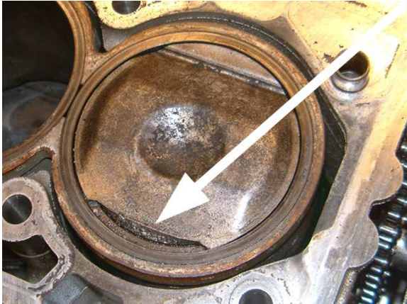
Figure 7: Damaged piston due to high PCP
