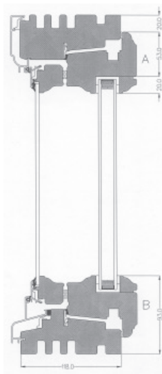
Figure 2.6 Example of window from the second round of the technology procurement program with total U -value of 1 \text{W}/\text{m}^2\text{K} . The triple glazing consisted of: 4 mm LE – 70 mm Air – 3 mm – 15 mm Ar – LE 3 mm.
