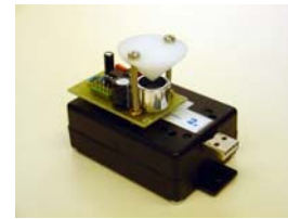
Fig. 2. Stationary sensor network nodes with ultrasound receiver circuit. The node is packaged in a plastic box to reduce wear.
