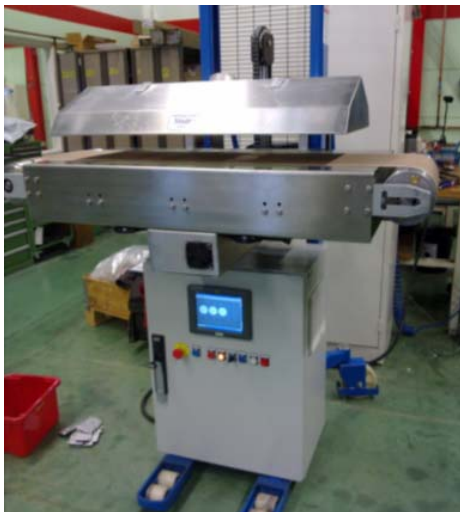
Figure 6. Evaporator using the Greenheat induction heating technology to heat the workpieces coming from a press operation.
