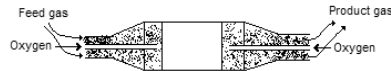
Fig. 1: Reactor setup with two heat buffers, each with its own oxygen inlet.
