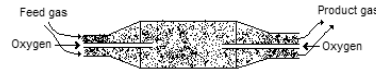
Fig. 2: Reactor setup with a fully packed bed with two independent oxygen inlets.
