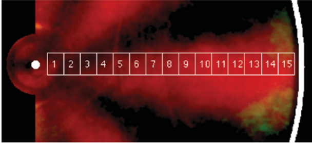
Figure 6. Visualization of the binning zones used for the spectral evaluation of the formaldehyde/PAH LIF along the jet axis.
