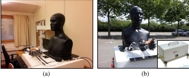
Fig. 1. Channel measurement receiver setup – (a) indoor in one-hand mode; (b) outdoor in two hands mode and Maury MT982EU30 tuner.
