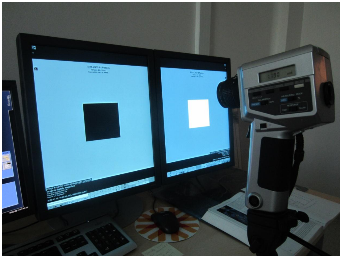
Figure 1. Measurement of maximum and minimum luminance with a telescopic photometer. In this paper, results from measurements of only one of the monitors are presented.
