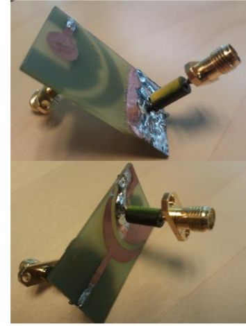
Fig. 17. The ferrite rings on the feed cables.
