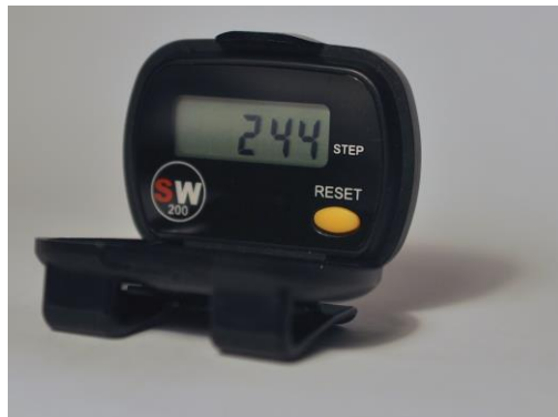
Figure 1. The pedometer (Yamax SW 200) used for measuring the number of steps in Study I-III.
