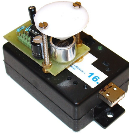
Figure 4. Stationary sensor network nodes with ultrasound receiver circuit. The nodes are packaged in a plastic box to reduce wear.
