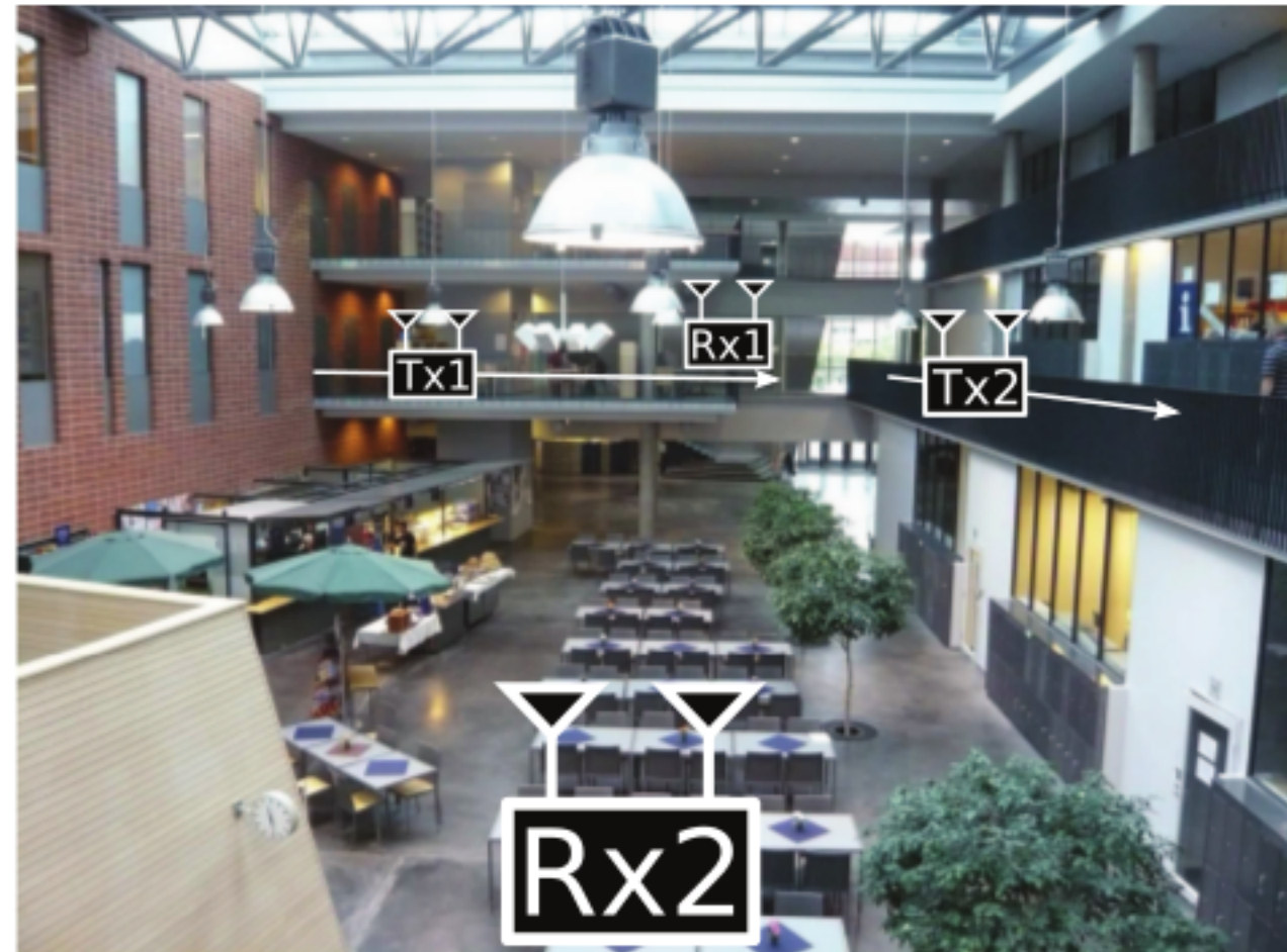
Fig. 4. Photograph of the measurement location. The receivers (Rx1 and Rx2) are static, while the transmitters (Tx1 and Tx2) move along the paths indicated by arrows.
