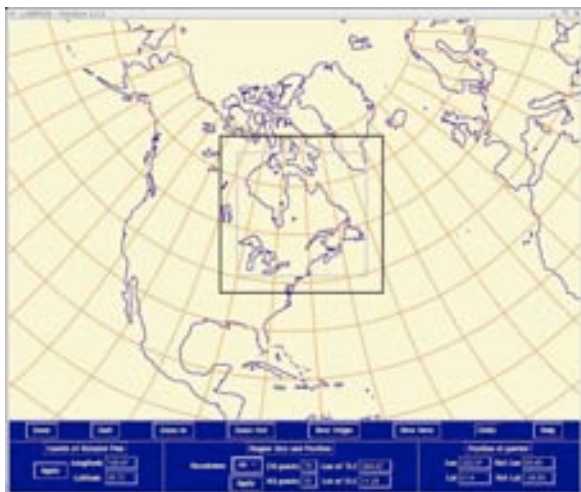
Figure 1. Defining the experimental domain on an interactive control panel; to ensure that PRECIS grid boxes are quasi-regular in area, the coordinate pole of the lat-lon RCM grid is rotated and placed over the centre of the domain.
