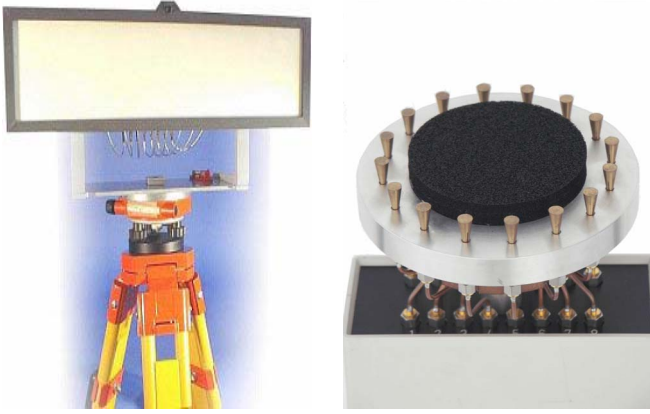
Fig. 1. An 8-element dual polarized uniform linear patch array was used at the transmitter side and a 16-element vertical polarized uniform circular array was used at the receiver side.
