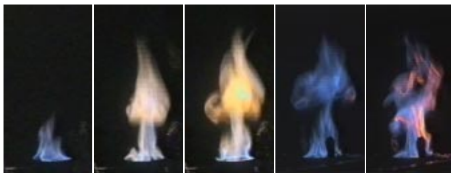
No ext. agent HFC blend A at 80% of ext. conc. HFC blend A near extinction HFC-227ea at 80% of max. conc. HFC-227ea at max. conc.
