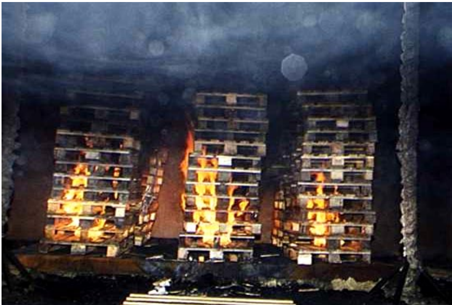
Figure 6. Fuel arrangement in the tests described in Paper V. The front row of pallets was sufficient to prevent water from reaching the row of pallets behind.
