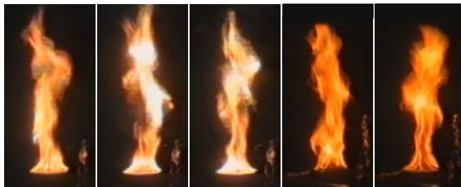
No ext. agent HFC blend A at 80% of ext. conc. HFC blend A near extinction HFC-227ea at 80% of ext. conc. HFC-227ea near extinction
