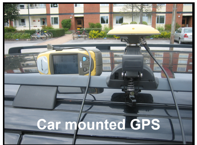
Fig. 6. High accuracy GPS with an external antenna mounted on the top of the car.
