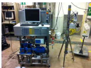
Figure 7. A pilot scale chromatographic skid, consisting of control software, pumps and valves, and a dynamic axial compression column.
