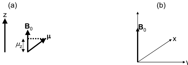
Figure 3.2 (a) The interaction of the static magnetic field with the magnetic moment, and the projection of the magnetic moments z component onto \mathbf{B}_0 . (b) Coordinate system defined according to the time independent static magnetic field, \mathbf{B}_0 .
