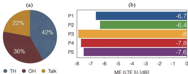
Fig. 7. (a) Relative usage in TH, OH and Talk modes, (b) usage-weighted ME.
