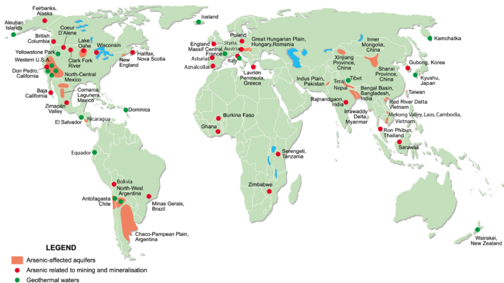
Figure 1: World-wide documented distribution of arsenic in ground water (>50 µg/L), related to mining and geothermal activities. Reproduced with permission of the British Geological Survey © NERC. Smedley, P. L. and Kinniburgh, D.G. 2013. Chapter 12: Arsenic in groundwater and the environment. In: Essentials of Medical Geology , Second Edition. Eds: Selinus, O., Alloway, B., Centeno, J.A., Finkelman, R.B., Fuge, R., Lindh, U. and Smedley, P.L. Springer, pp 279-310. ( http://www.bgs.ac.uk/about/copyright/acknowledgements_published.html ).
