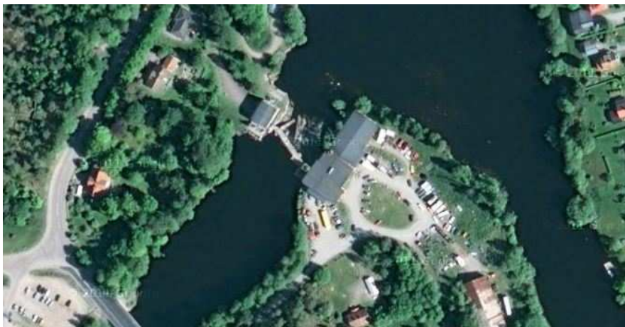
Fig. 1 Plan view over from left to right: the power plant, spillways, workshop building and embankment dam (from Google maps).
