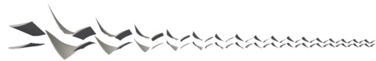
Figure 3: Geometric design of the compressor gas path seen from the top (radial X-Z view).
