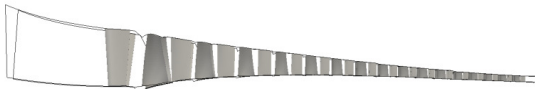
Figure 2: Geometric design of the compressor gas path seen from the side (X-Y view).
