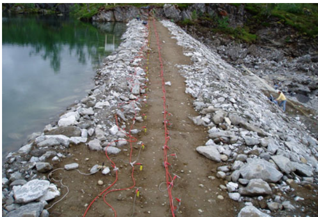
Fig. 7 Electrode layout along the dam crest at the Rössvatn test embankment dam, with non-polarising Cu-CuSO 4 electrodes for SP monitoring to the left and stainless steel electrodes for resistivity and IP monitoring to the right
