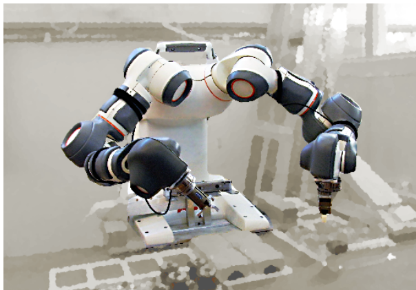
Figure 2.1 ABB YuMi Robot [ABB Robotics, 2015; Kock et al., 2011] used mainly for experiments in Sections 2.2 and 2.4.
