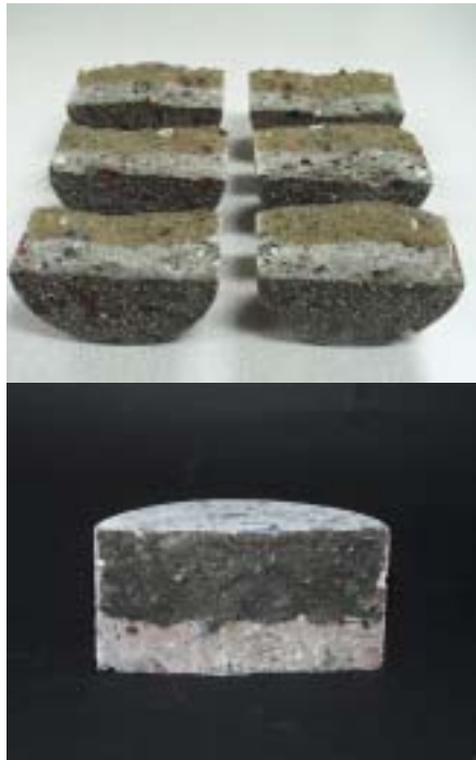
Figure 19 - The chloride penetration depth determined by measuring three cut specimens with silver nitrate [67].
