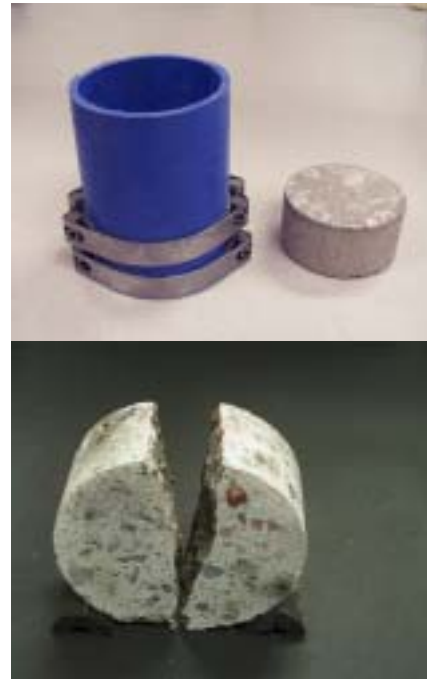
Figure 18 - A rubber sleeve assembled to the specimen that was cut afterwards.
