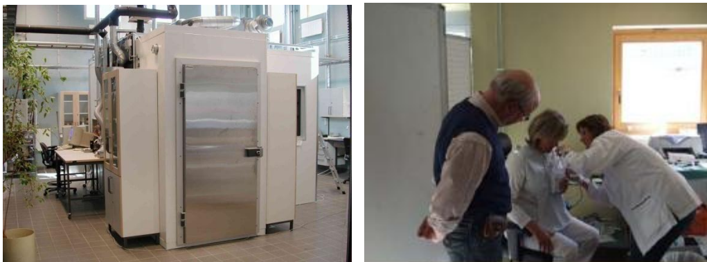
Figure 4. Left: a walk-in chamber at Lund University, Sweden, where extensive studies are performed on how indoor environmental factors affect humans. Right: one of the test persons is examined after being exposed to airborne particles in the chamber.
