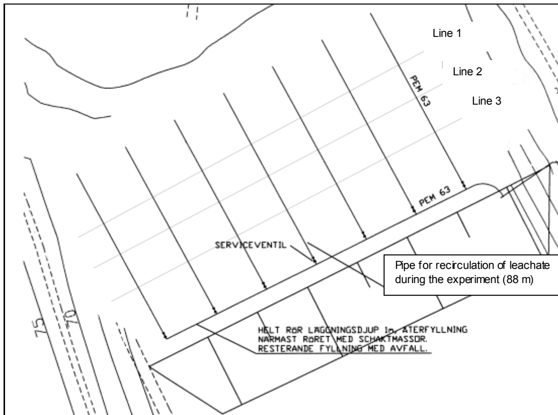
Figure 1. Plan of the bioreactor landfill showing the distribution pipes for leachate and the lines for resistivity measurements (Line 1 – 3)
