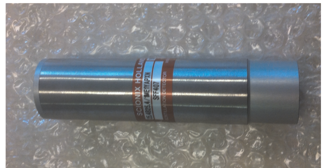
Fig. 2. Photograph of a YAP detector. A 1 in (diameter) \times 1 in (height) crystal has been mounted on a 1 in (diameter) \times 10 cm (length) PMT.
