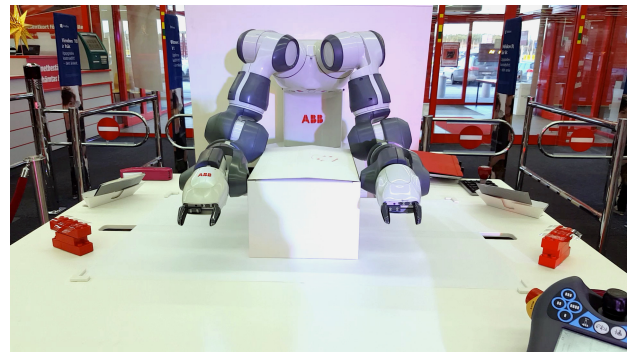
Fig. 3. The position of the package was fixed by squeezing it between the arms.
