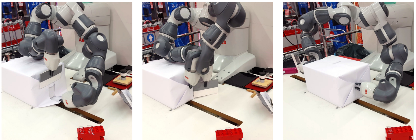
Fig. 7. The folding of the short side. Left: The incision in the table top was used to pick up the bottom flap. Center: The lower flap was handed over to the holding arm to enable the taping. Right: The holding arm was moved to the other side of the package to fixate it when the tape was attached.
