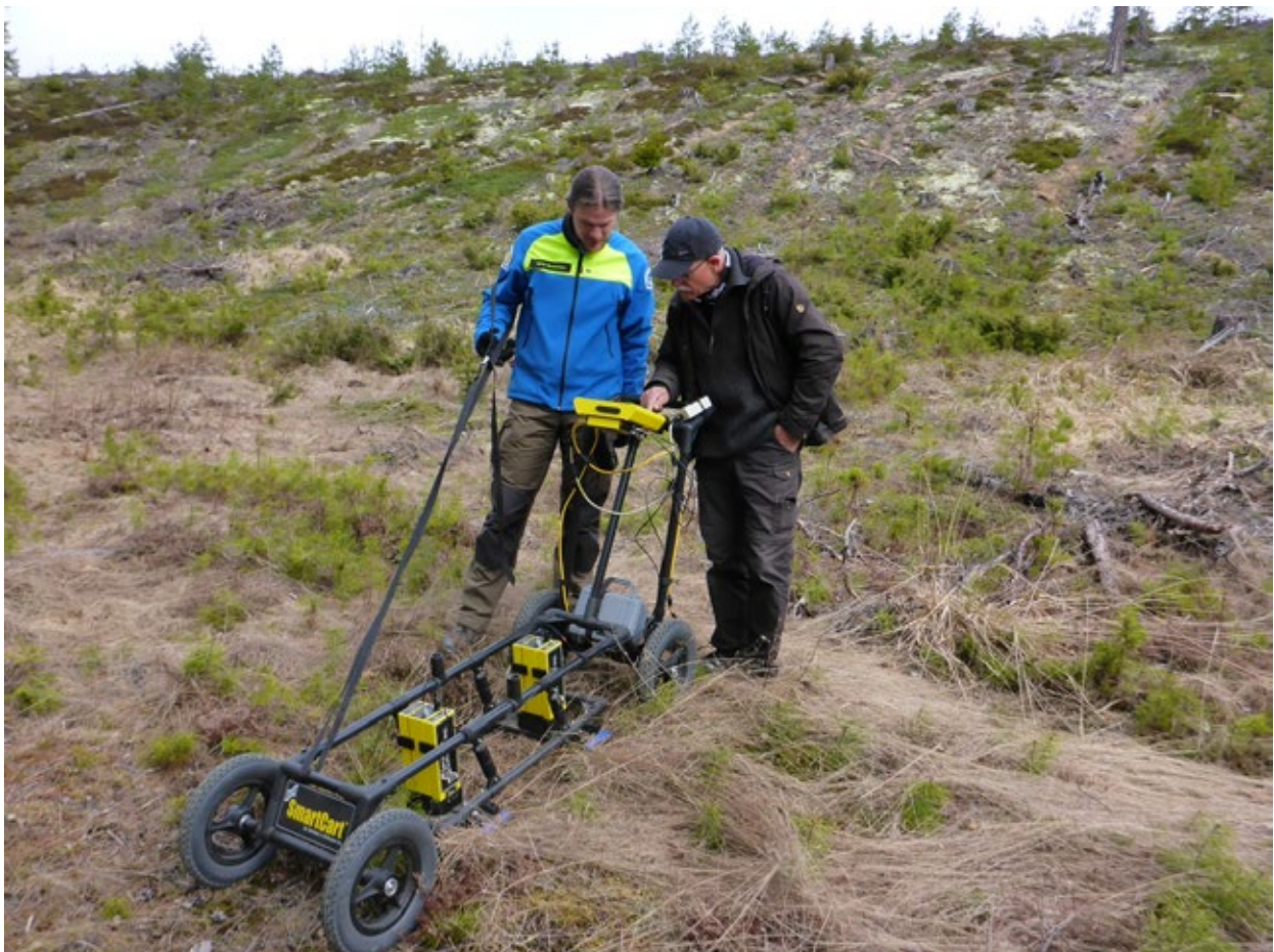
Fig. 4. Martin Bernhardson and Leif Jakobsen review the results of a GPR profile across the dune at Orsa 3 in Dalarna.
