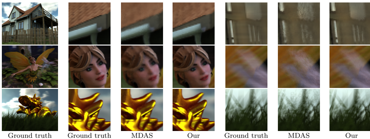
Fig. 13 Image quality comparison for equal time renderings. The noise in our images is greatly reduced compared to MDAS. The images are rendered with 16k initial random samples, after which adaptive sampling kicks in. Top: House scene (93.6k tris) after 676s rendering with our algorithm and 712s with MDAS. Middle: Fairy scene (194k tris) after 504s with our algorithm and 519s with MDAS. Bottom: Dragon scene (301k tris) after 4114s with our algorithm and 4973s with MDAS.
