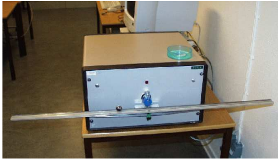
Figure 10.2 The ball and beam process.
