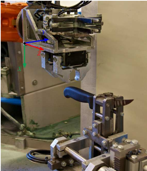
Fig. 2. The knife reorientation station and the knife gripper mounted on the robot. The orientation of the robot flange coordinate system is also shown.
