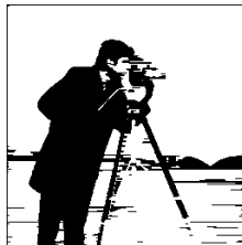
Figure 8.3: Result using CUDA Cuts (Vineet and Narayanan, 2008) with \rho = 10^4 . The correct solution is shown in Fig 8.2. For \rho = 10^5 and 10^6 the algorithm produces a constant image.
