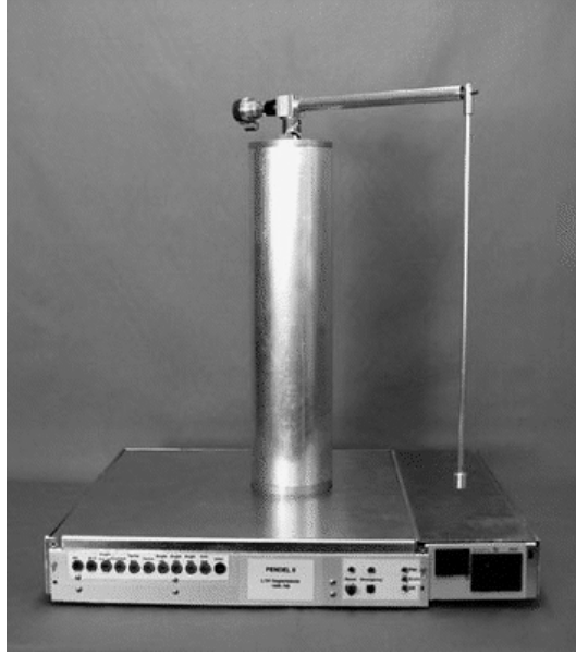
Figure 3.6 Furuta pendulum, Department of Automatic Control, Lund.
