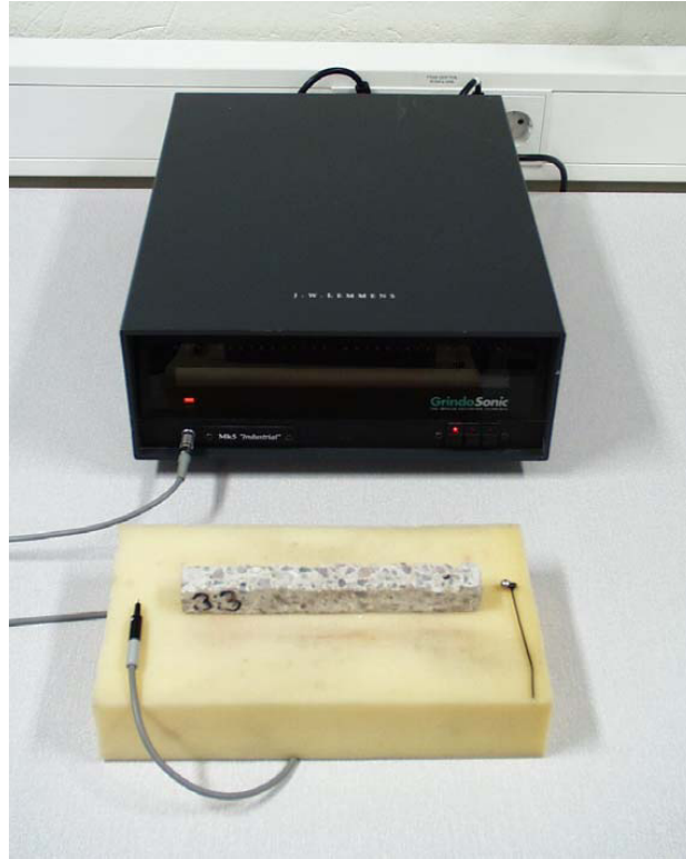
Figure 4.4.5 Equipment for measuring the resonance frequency.
