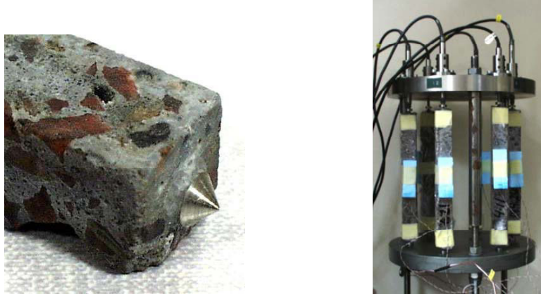
Figure 4.4.1. The test set-up for measurement of changes in length.
