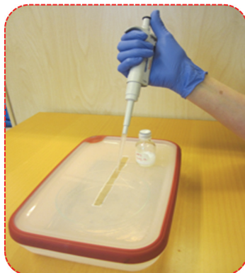
Transferring a mixture of VOCs to a container
